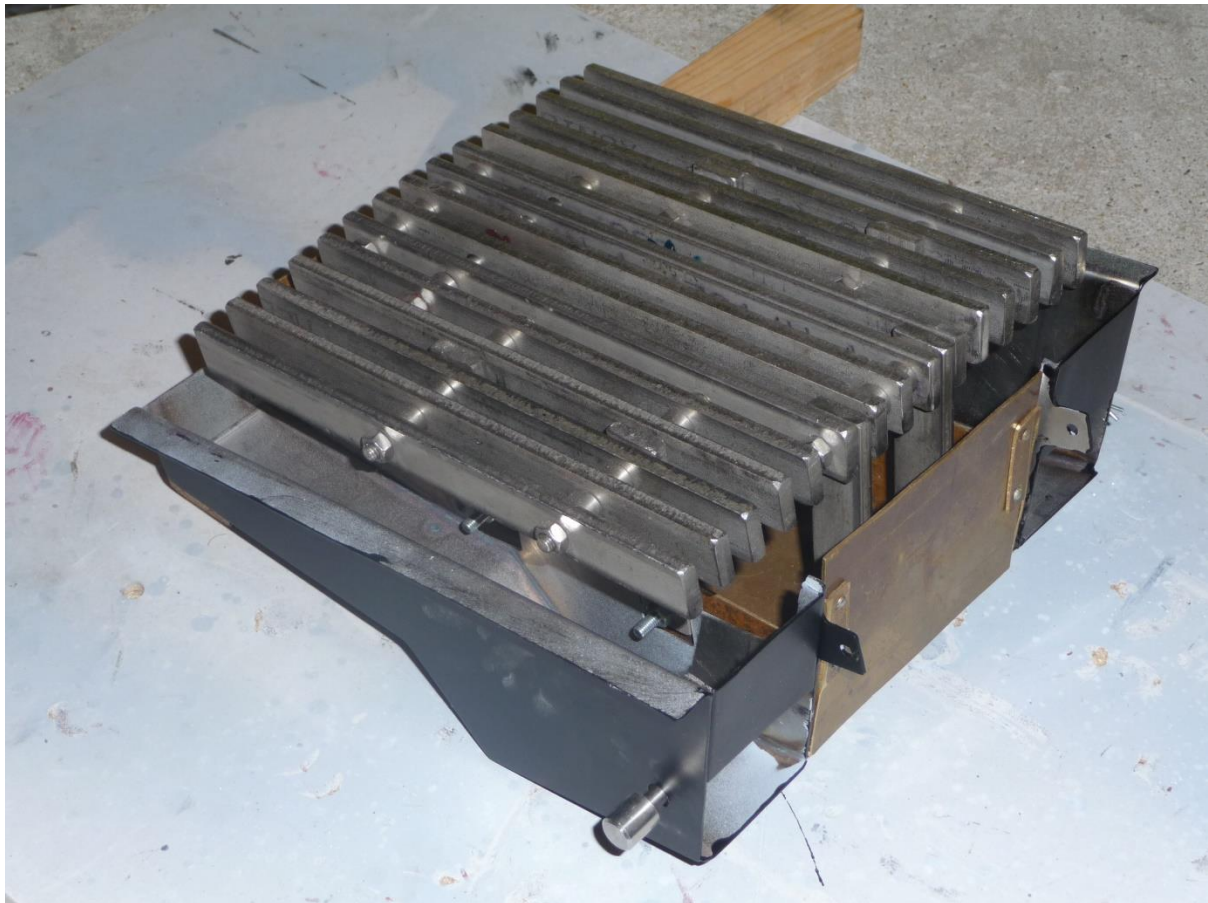
Fig 11: Ashpan and Grate – the centre section of the ashpan is brass, everything else is stainless. The end of the long pin (used to drop the fire) is visible at the bottom of the photograph. The centre section of the grate can be completely removed when needed.
