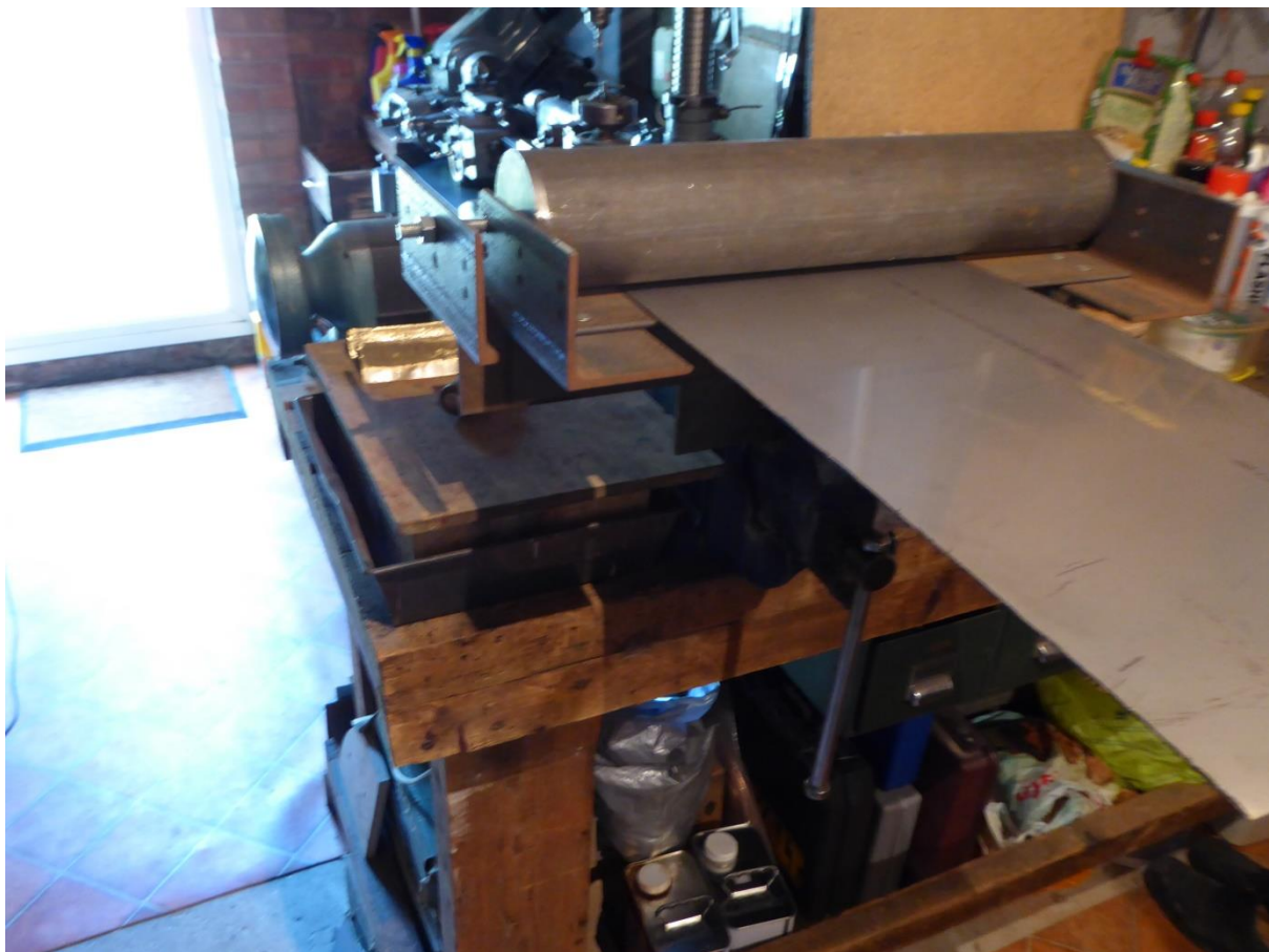
Fig 10: Preparing to bend the outer firebox cleading on the modified simple bending machine – a long lever is located beneath the sheet metal and a good upward push ‘rolls’ the metal round the tube visible at the top of the picture.
