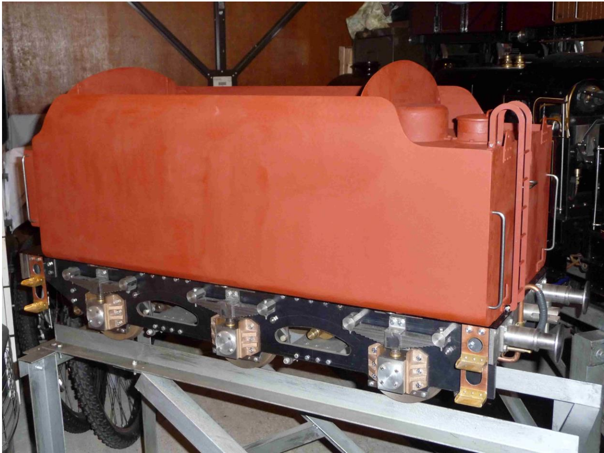
Fig 4: The completed tender awaiting final painting – it is about 1½” longer as a result of stretching than a normal BR1C tender. The vacuum release valve is just visible between the centre and rear axles.
