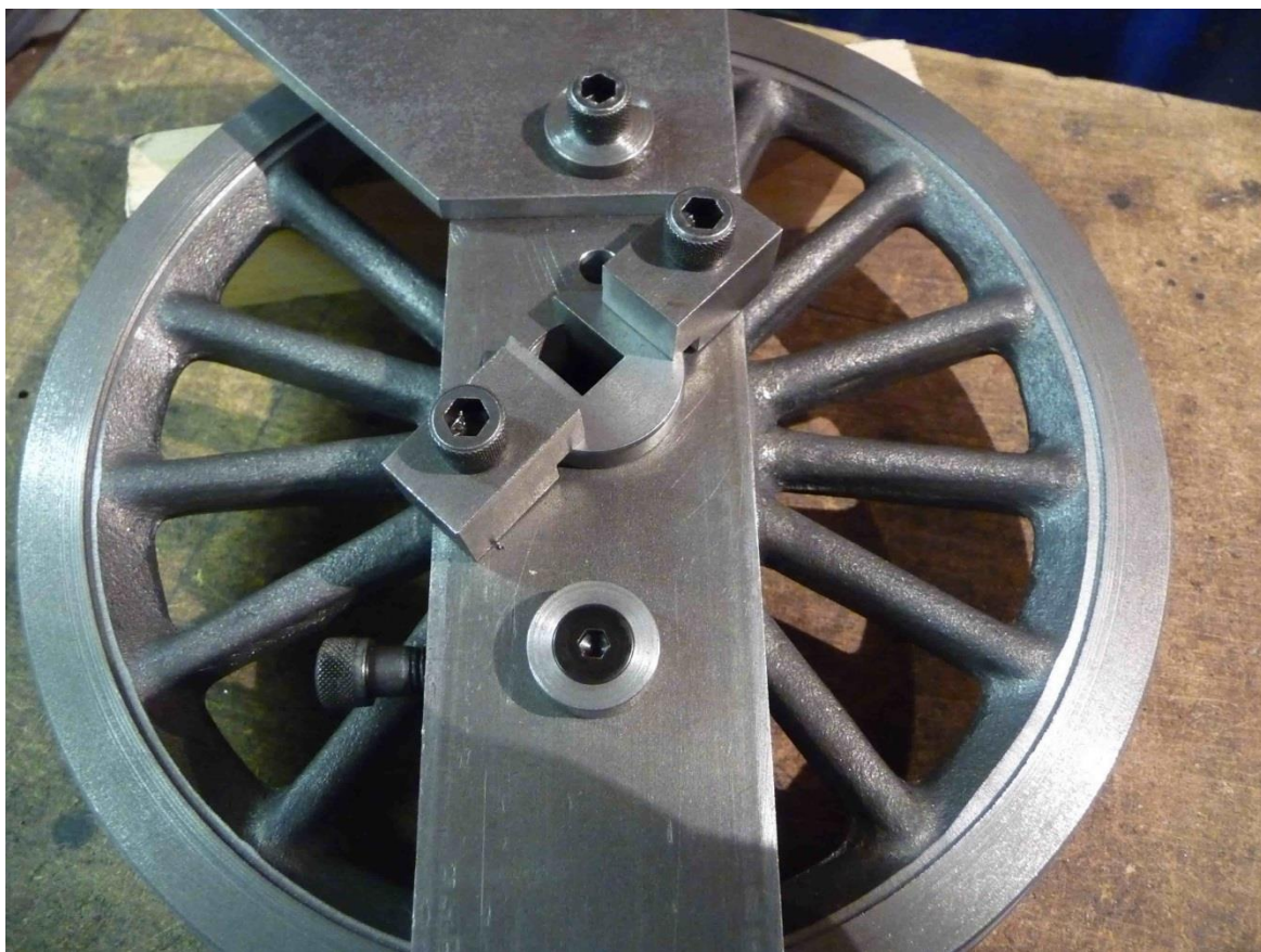
Fig 5: The Quartering Jig. The broaching bush goes into the axle bore and is held by the jig which is located by the pin in the crankpin bore (nearest the camera). The keyway is cut at 45°, with the angle of the broaching bush being set by the plate visible at the top, using a piece of the ¼” keyway steel (that will be used to make the keys) fitted into the broaching bush slot. A keyway in the jig is also cut at the same time as that in the first wheel (after this photograph was taken) which helps repeatability. The main part of the jig is made out of 12mm bright steel bar, by the way.
