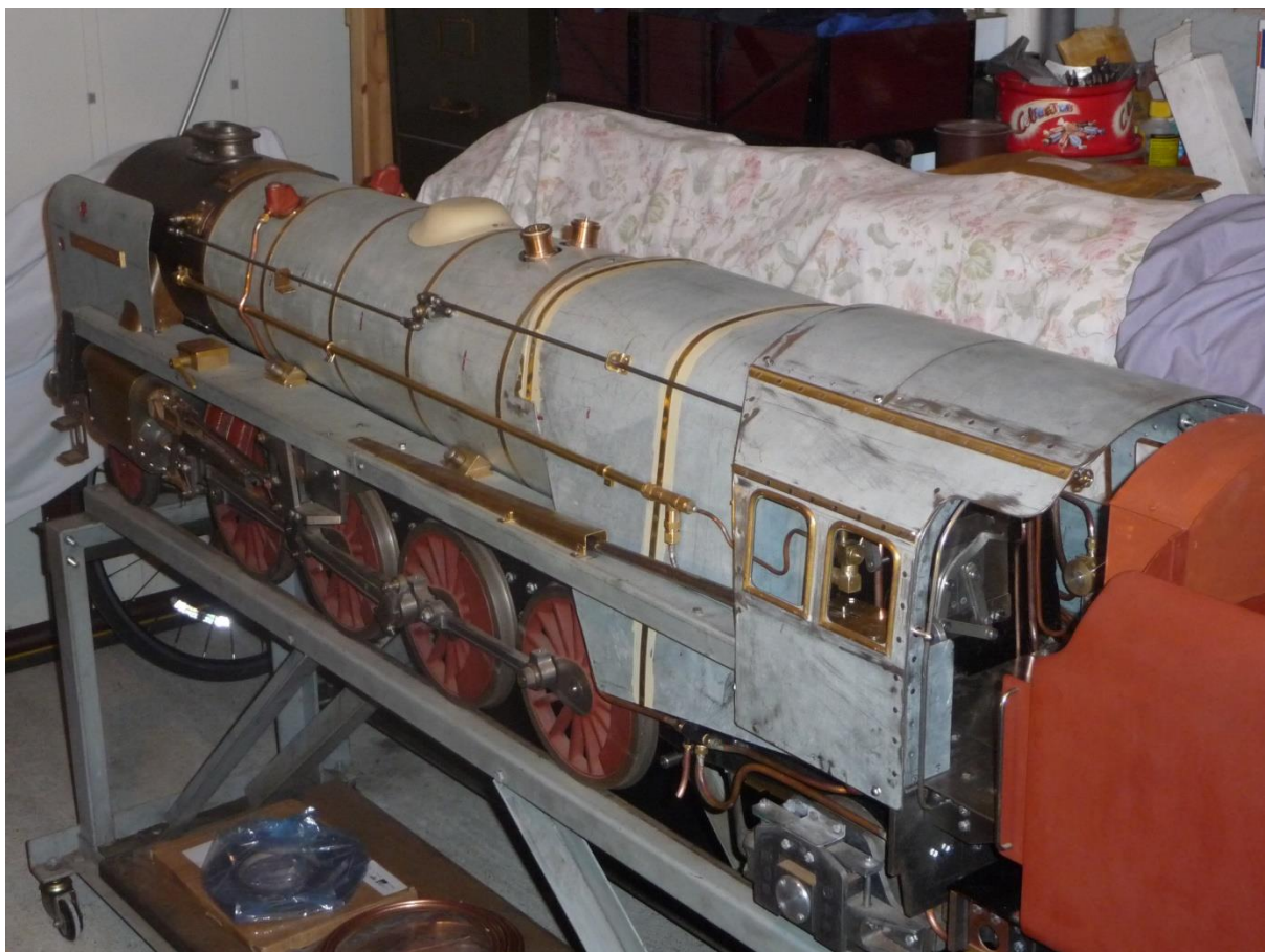
Fig 12: Nearly finished, just a few parts to make and a lot of painting still to do in March 2017. Hopefully the firebox cleading is like the original might have been. Note the tidy appearance just ahead of the cab roof – no pipes.
