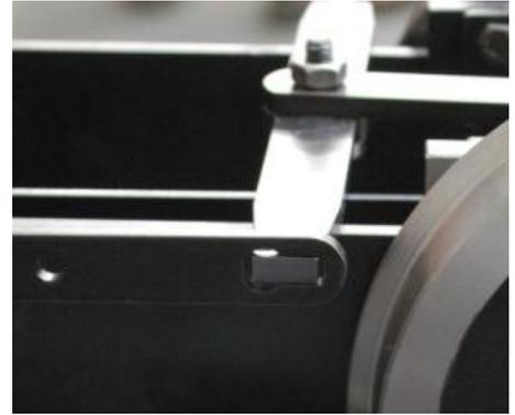
26. Attach a brake shoe to each brake hanger using an M6 x 20mm CSK bolt and nyloc nut as shown.
