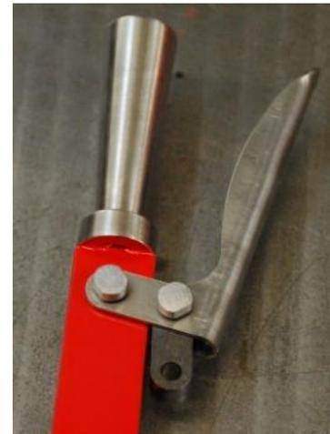
90. Attach the reverser latch lifting links to either side of the reverser lever latch using M4 x 20 motion pins as shown, ensure that the holes used in the reverser latch lifting links are the ones at the end of the shorter shafts so that the remainder of the part can be situated so that it is parallel with the Reversing lever, attach via a M4 x 20mm motion pin, from the front and nyloc nut.
