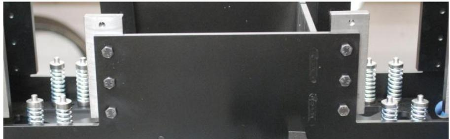
9. Using a 3mm Allen key, loosen off the two Allen screws on each axle bearing, so that the bearings will move up and down freely.
