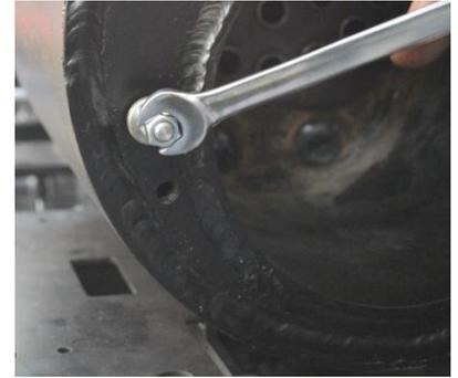
125. Fit the pair of injector clack valves as shown, using Loctite 243 to seal the threads. Make sure the pipe unions face downwards.
