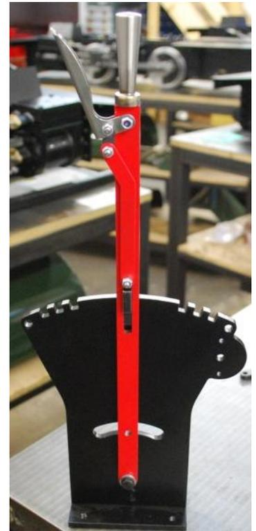
93. Grease the reverser lever spacer and push it through the large hole in the reach rod. Fix to the reversing lever as shown using an M6 x 30 hex head bolt and nyloc nut - the nut runs in the slot in the stand, bolt
