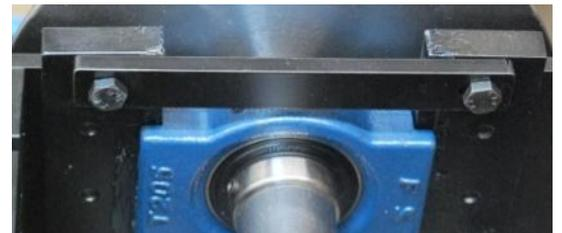
13. Set the rear axle in its correct position by pushing it hard up against the rear hornblocks - this is the pair that have previously been fully tightened. Push the front hornblocks back against the rear axleboxes and tighten up both sides - check that the axleboxes slide freely up and down the full length of the hornblocks.
