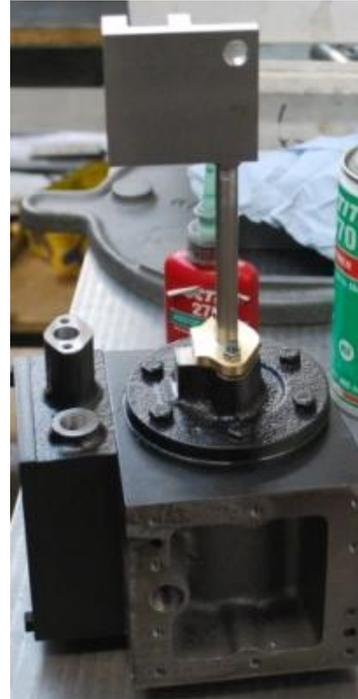
31. Run an M8 half nut down the piston rod, then fit the right hand crosshead - don't tighten the nut at this stage.
