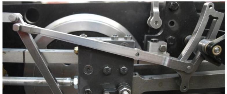
85. Connect the lifting link to the radius rod using an M4 x 20 motion pin and nyloc nut as shown.
