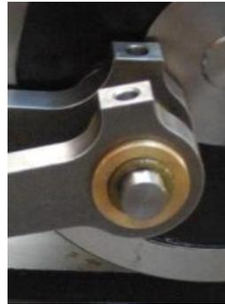
58. Fit the connecting rod, flange of the big end bush faces outwards, oil well at the crosshead end faces upwards as shown.
