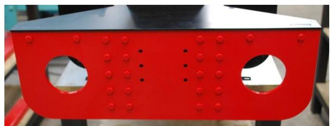
110. If not previously assembled, attach drag beam and buffer beam to the chassis. The buffer beam has two large holes in it to allow removal of the pistons for maintenance. Attach using 24 off M6 x 16mm hex head bolts, fit to all the holes except the six coupling mounting holes shown in the middle of the Beam. Attach the drag beam in the same way using 24 off M6 x 16mm hex heads to the twenty four holes except from the six inner holes.
