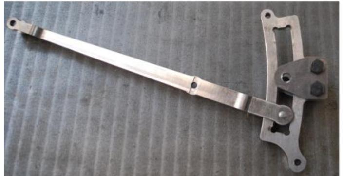
81. Fix the expansion link trunnion pins as shown using Loctite 243 - hold in a drill or lathe chuck to tighten.
