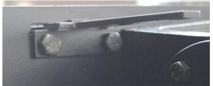
41. Bolt drain cock cross shaft to the operating lever using two M5 x 12mm hex head bolts and nyloc nuts.
