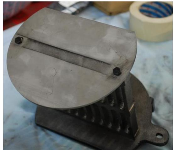
Attach baffle to the grate as shown, using a pair of M6 x 20 bolts - cut off bit goes to the top, round bit to the bottom.
