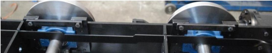
39. Slide the drain cock cross shaft through the slots in frames just in front of the cylinders as shown.
