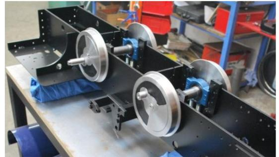
12. Loosely bolt the hornstays across the four pairs of hornblocks using M6 x 16mm hex heads, slotted hole faces the front of the engine.
