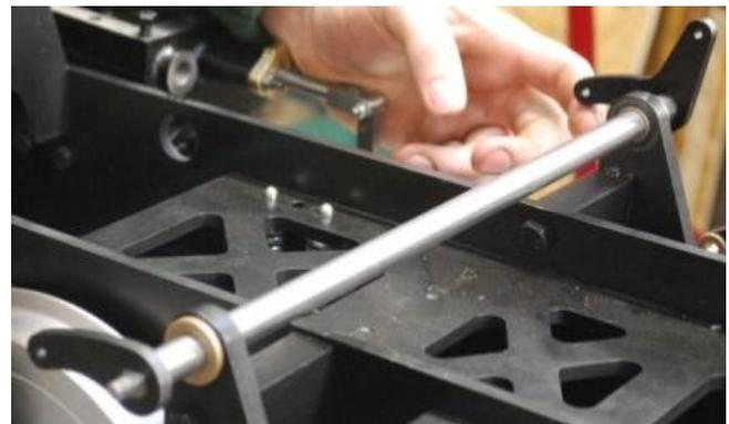
77. Fit combination lever to the valve spindle clevis using an M4 x 20 motion pin and nyloc nut. The combination lever has three holes in it, the two closest together are at the top - the machined notch between these holes faces the front of the engine.
