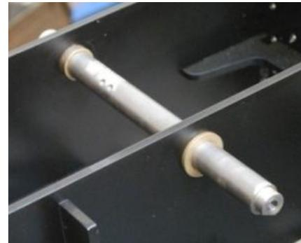
22. Fix the brake link centre to the shaft with an M6 x 10mm grub screw, fitted with Loctite 243 - ensure that the screw engages with the dimple drilled in the shaft.
