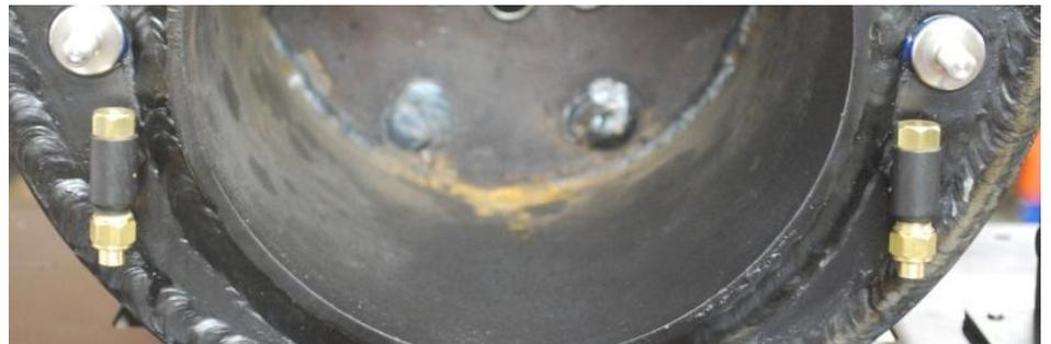
126. Fit the injector delivery pipes to the clack valves as shown, one each side.
