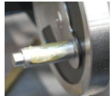
16. Turn the wheels so that the crankpins are at the front dead centre position as shown. Using a square, set the front axle's front hornblock square with the bottom edge of the frames and tighten its three securing bolts with the hornblock lightly pushed up against the axlebox. Turn the wheels to back dead centre, push the rear hornblock up against the axlebox and tighten its fixing bolts.
