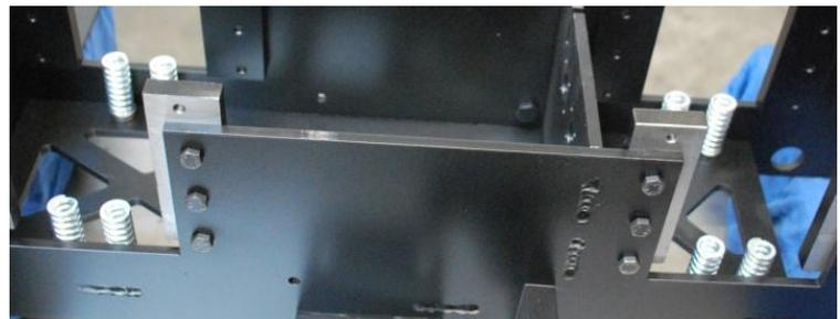
8. Fit bottom spring platforms onto the springs - again the thick ones go on the rear axle, thin ones on the front.
