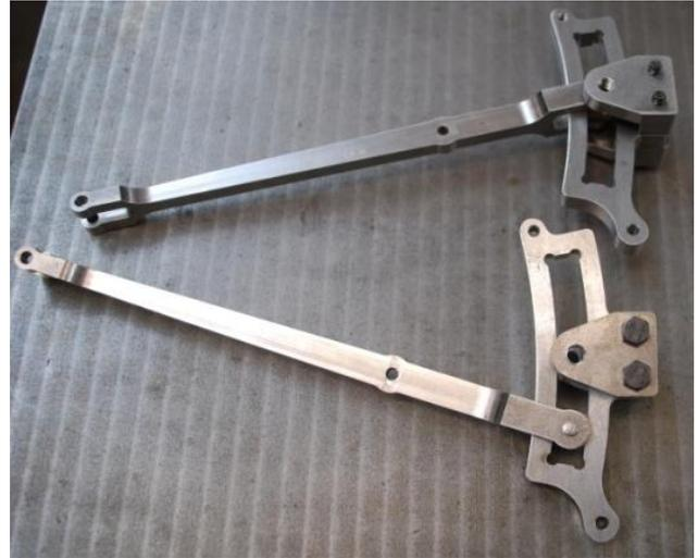
83. Remove the motion bracket outer plate. Lightly oil the expansion link trunnion pins and fit as shown - refit outer plate and tighten the bolts. Make sure that the expansion link can swing freely.
