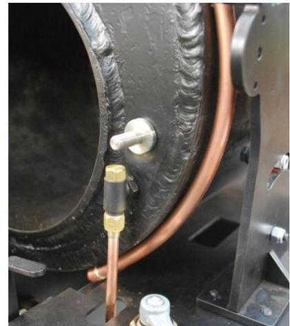
147. Fit 10mm unions to each valve chest using PTFE as shown. Fit the left hand steam pipe (longer one) into its union in the left hand valve chest, right hand (shorter one) to the right hand steam chest.
