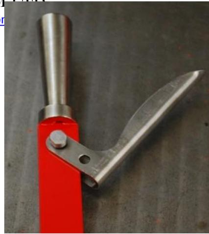
89. Attach the reversing lever trigger link using an M4 x 15mm motion pin as shown. grease on assembly.
