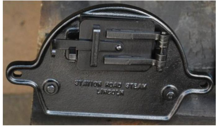
This is quite a good time to paint the Backhead - it's the one part of the whole engine that gets seriously hot and needs some very high temperature paint to have any chance of staying on. We use barbecue paint in an aerosol.
