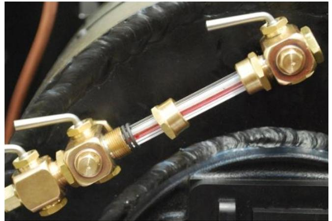
155. Fit the water gauge blow down pipe as shown - bottom end goes through a small hole in the left hand footplate, next to the injector water valve.
