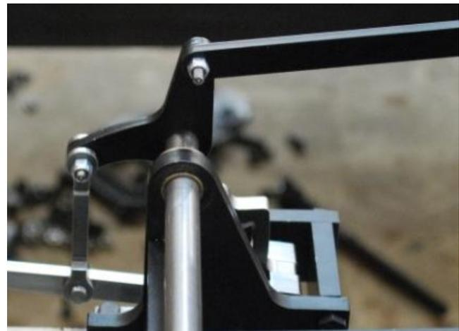
96. Set reverser into full forward gear and observe the position of the die block in the expansion link ( it will be towards the bottom). Now set it into full reverse and again check the die block - it will be near the top. The aim is to end up with an equal gap top and bottom in reverser and forward gear respectively - to adjust, slide the complete reverser stand backwards or forwards along the footplate. When set correctly, tighten the four mounting bolts fully.
