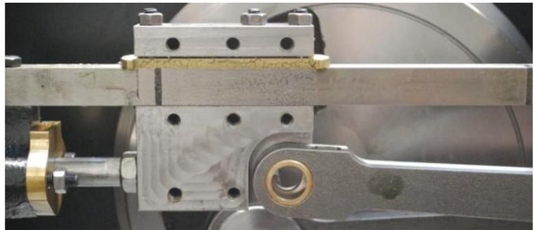
59. Remove crosshead cover plate, grease the gudgeon pin, then refit the cover, ensuring that the gudgeon pin slides easily through the connecting rod bush.
